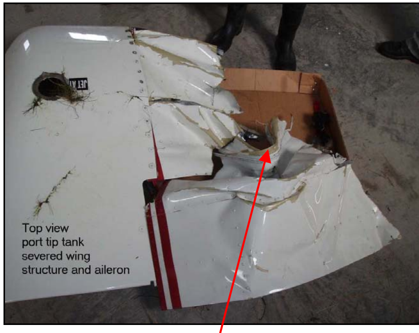
Photo No 1. Indentation made by tree
